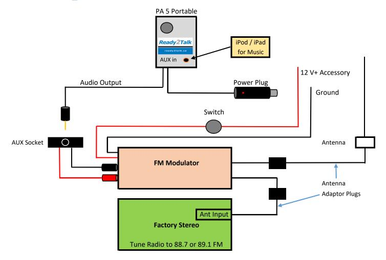
The TAK connects the PA to the antenna circuit of your factory stereo through the FM radio using a FM Modulator. Once connected, to use the PA just turn the on/off switch and it will in turn activate the FM Modulator. Next put your stereo into the FM radio mode and tune into 88.37 or 89.1 MHz and you will hear the PA.
