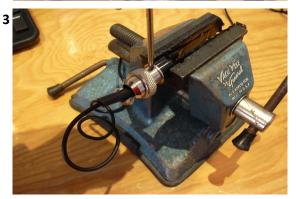
Remove locking screw Pull back metal clamp assembly
