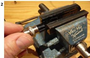
Put mic plug into vise with notch facing you Tighten Vise
