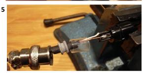
Problem B Wires pulled and can short when assembled
