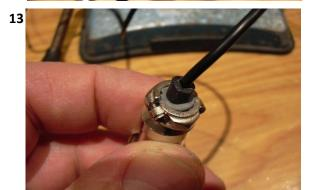
The rubber grommet should be pushed in completely
