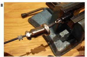
Slide the metal clamp assembly on to the plug and screw tight
