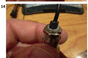
Tighten metal clamp screws Test operation
