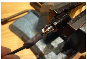
Re-solder wires back on plug #1 Braided wire #2 White Wire
