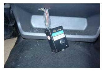
**Step 5** Using crimp connectors, connect the red wire on the PA to the gray and the black PA wire to the black with blue stripe. Fish the PA output wire and connect to the AUX input socket. Tape the connection to make sure it never comes undone.
