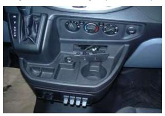
Step 2 Unclip the 3.5 socket assembly from the plate, you might need to insert a small blade to release the clips. Use caution!
