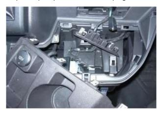
Step 4 Drill a 1" hole in the bottom of the console and fish the wires from the PA into the console area.
